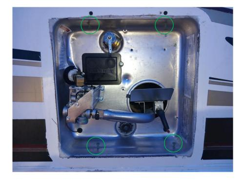
Add the <u>Butyl</u> tape to the perimeter of the frame and a bead of silicone, along <u>each</u> side of the Butyl tape.
