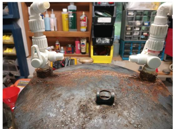
Install the valves on the new tank using Teflon tape on top of pipe dope.
